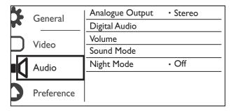
[Analogue Output] - Adjust this setting for audio output through AUDIO OUT L/R.
